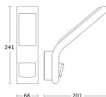
**Specifications Steinel LED Floodlight XLED Home Anthracite 10.5W 550lm - 830 Warm White | IP44 - Motion Sensor - Symmetrical**
